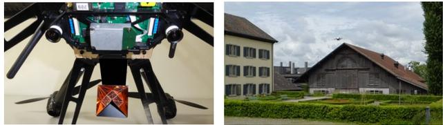
Fig. 5: The sensor system, providing visual (here we use only one camera) and inertial measurements, and a Leica prism underneath are attached to the AscTec Neo platform (left image). The garden environment, in which the first set of experiments have been conducted (right image).
