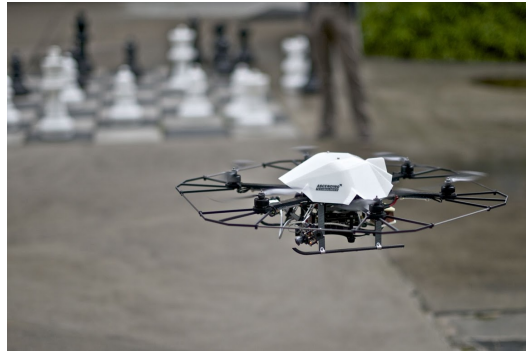
Fig. 1: The hexacopter which is used for the experimental analysis during an autonomous flight with the proposed framework
