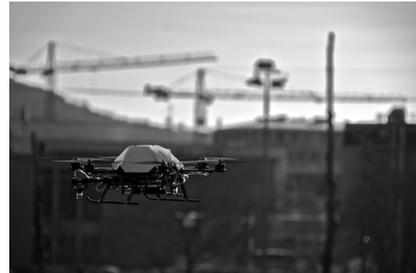
Fig. 1: Fusing information from the downward-looking camera and an IMU, the MAV performs SLAM in a disaster area
